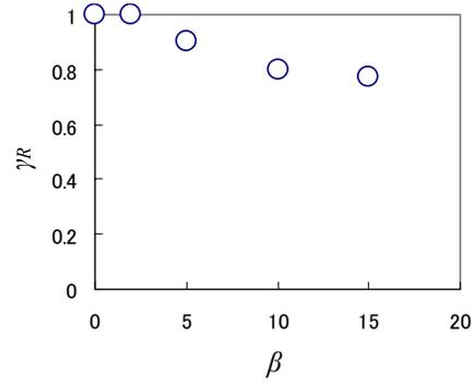
Fig.4 Decreasing ratio of inflow angle for rudder
