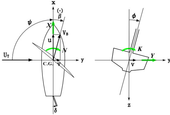
Fig. 3 Definitions of horizontal body axes system and angles
