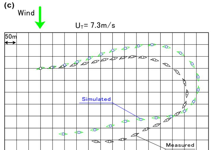
Fig. 7 Comparison between measured and simulated results at wearing maneuver (starboard tack to port tack)
