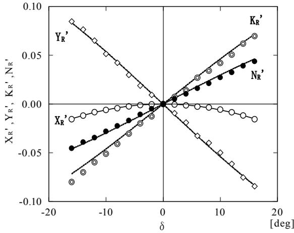
Fig.5 Variation of hydrodynamic coefficients of rudder with rudder angle  $\delta$
