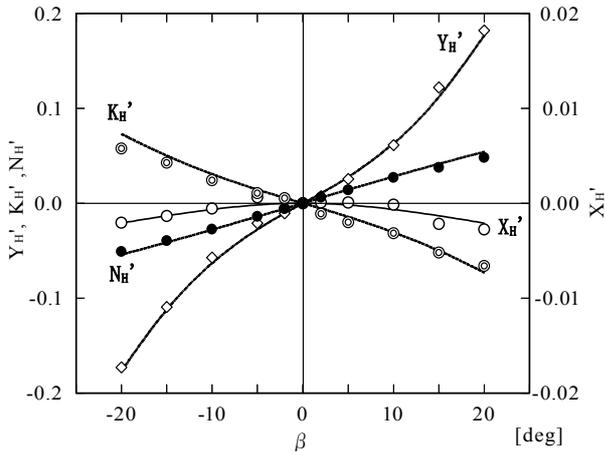
Fig.6 Variation of hydrodynamic coefficients of hull with leeway angle  $\beta$  (without rudder forces)
