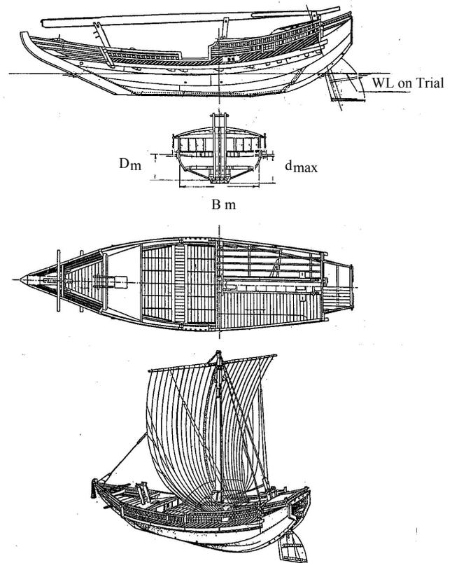
Fig.1 Arrangement plan of “Naniwa-maru”
